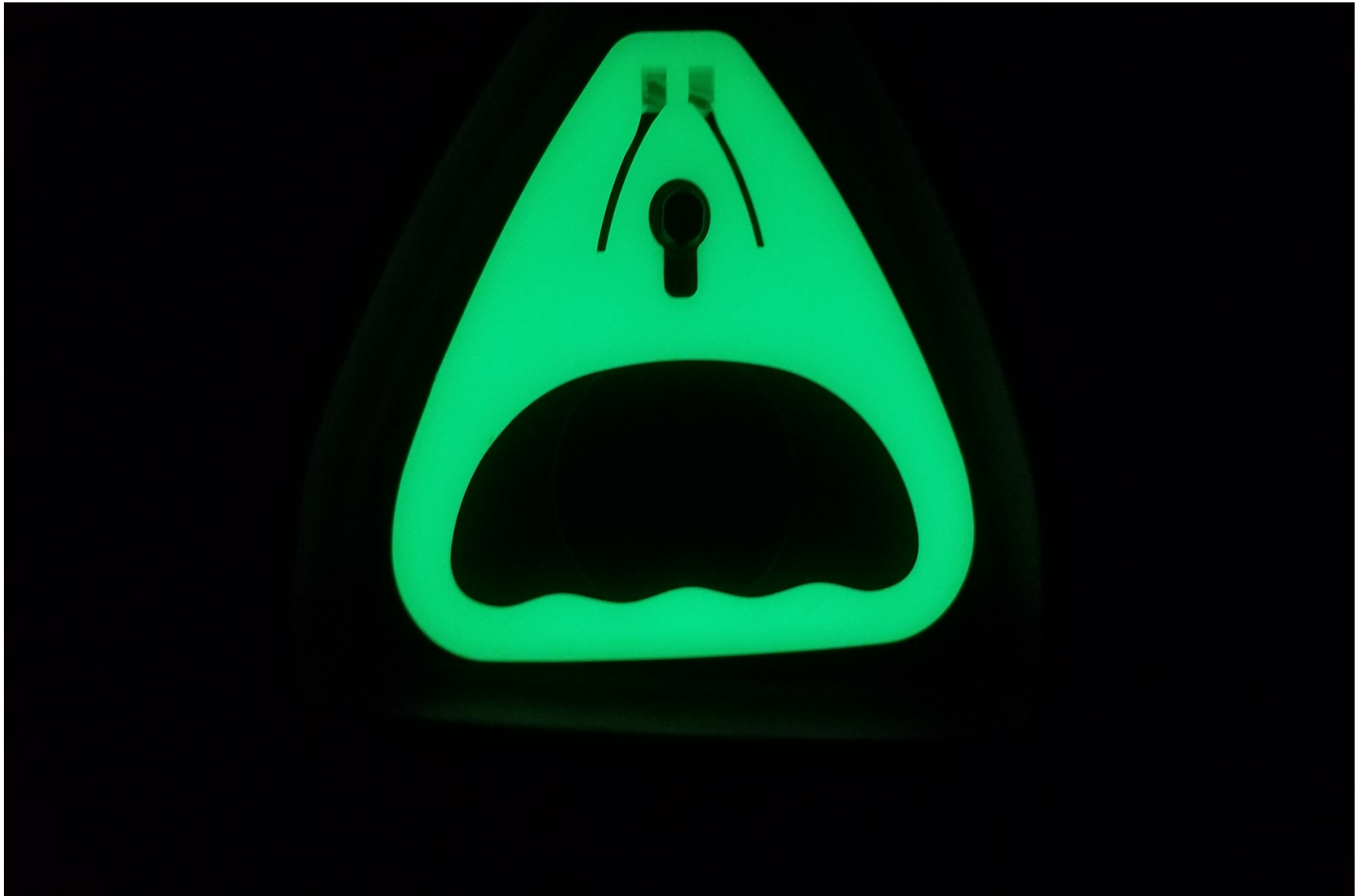
FIGURE 5.9 VEHICLE TRUNK COMPARTMENT MANUAL RELEASE MECHANISM ILLUMINATION
